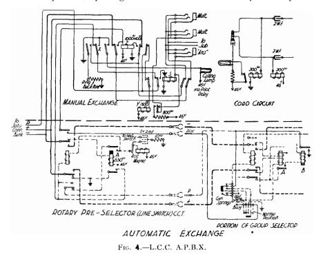
springs. In falling back it moves the wipers on to the next trunk. If this trunk is also engaged, the above cycle is repeated until an idle trunk is found.
