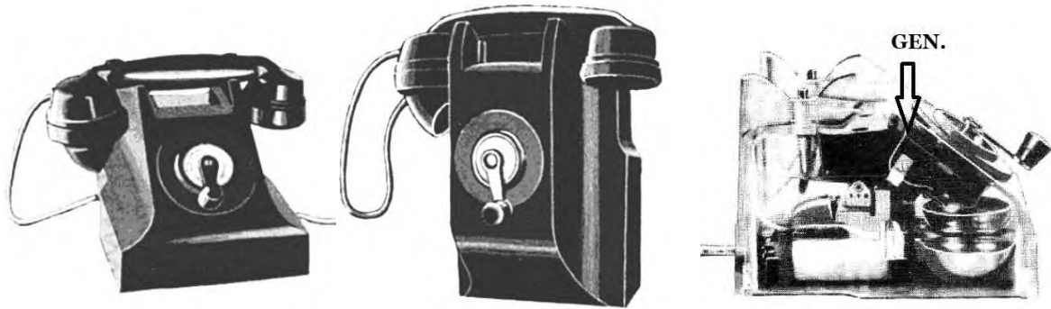
L-R: 300 MT, 300 MW, and generator location/layout
