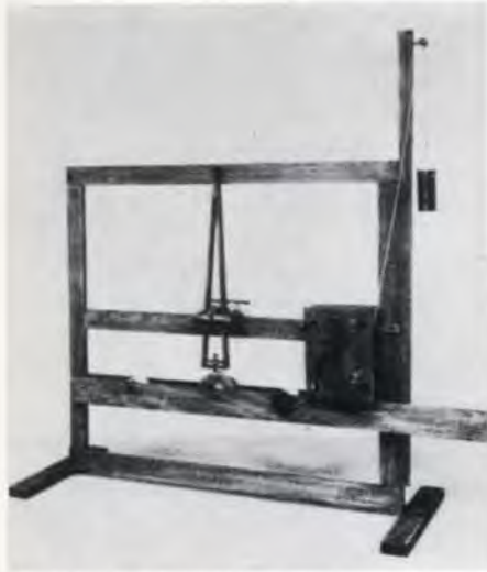
(Crown Copyright, Science Museum, London.) Fig. 7. Morse's electromagnetic telegraph. First model of the receiver, 1835 (replica).
