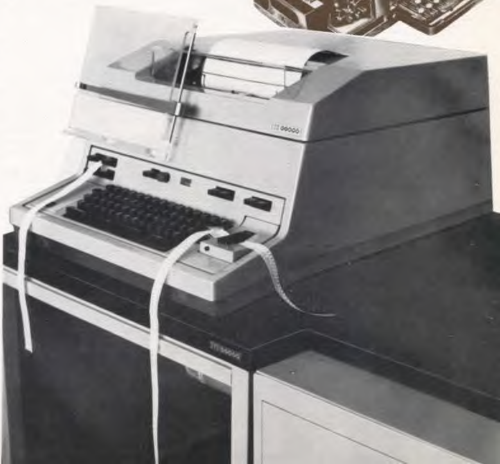
A Model 3 Tape Teleprinter, the first Creed machine produced as a combined start-stop transmitter receiver, in 1927, shadows a Model 444 Teleprinter, the current model in the ITT Creed range.
