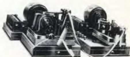
Fig. 10. Morse Reperforator and Morse Tape Printer
