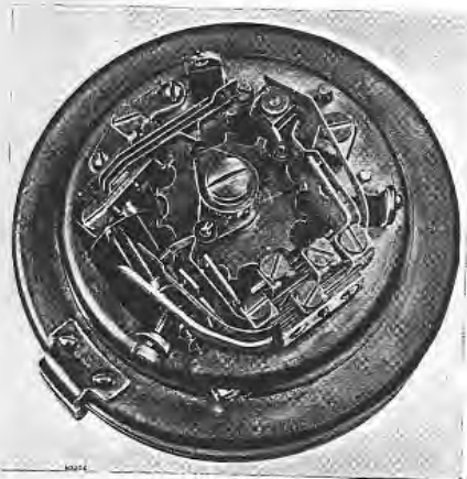
FIG. 14.—TRIGGER TYPE DIAL FOR USE WITH TESTERS
