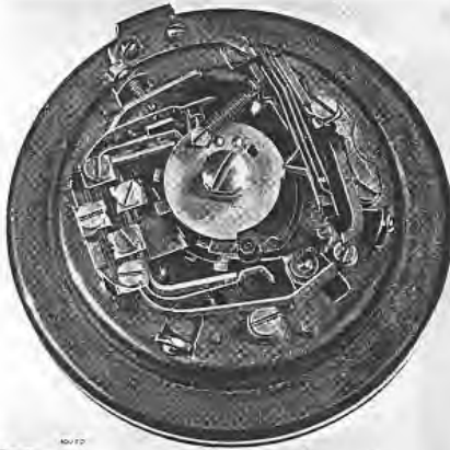
FIG. 13.—TRIGGER TYPE DIAL FOR USE ON COIN-BOX CIRCUITS—REAR VIEW
