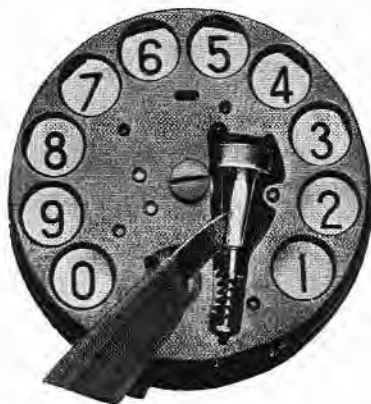
PLATE 3 see Paragraph 7.1 Method of adjusting governor wings.
