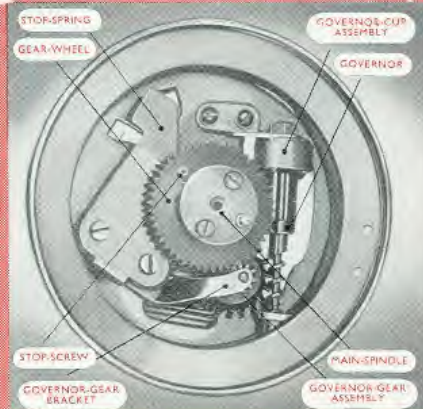
Driving and governor mechanism
