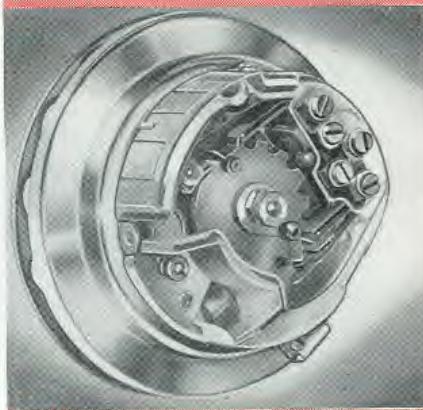
Rear View - assembled dial with transparent plastic cover.
