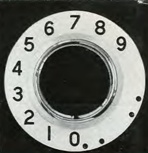
Number ring for rotary systems.
