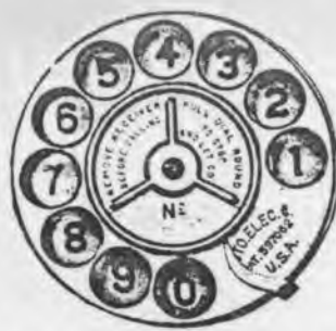
Fig. 12—A Later Form of Two-Wire Dial, the Forerunner of the Present Models—1911.
