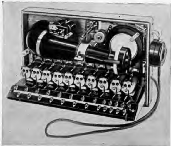
Fig. 604.—Interior of Dictograph Master Station, showing Arrangement of Loud Speaker.
