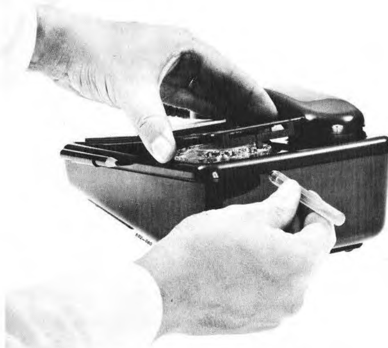
Fig. 3 — Method of Removing Faceplate
