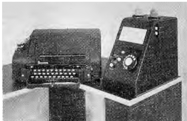
FIG. 11.- TELEPRINTER NO. 11B AND DIALLING UNIT.
