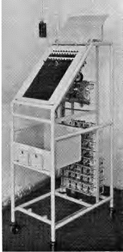
FIG. 25.—TESTER FOR TRUNK RELAY SET.
