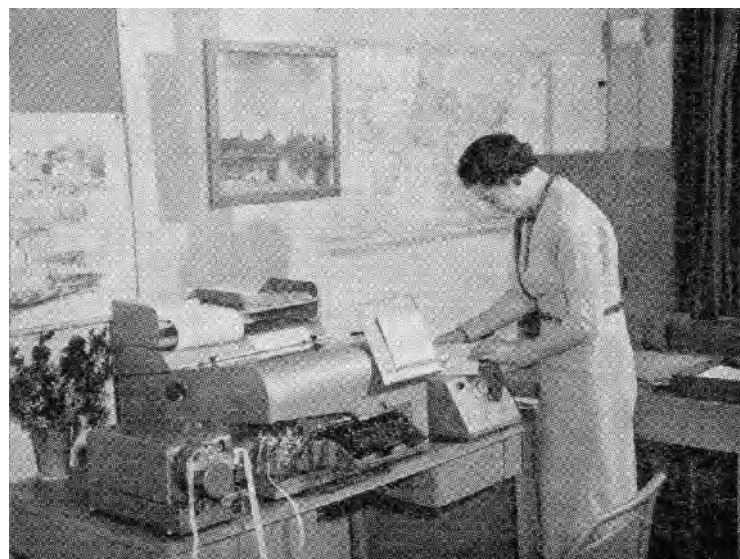
FIG. 14.—TELEPRINTER SET FOR STATION WITH AUTO TRANSMITTER.
