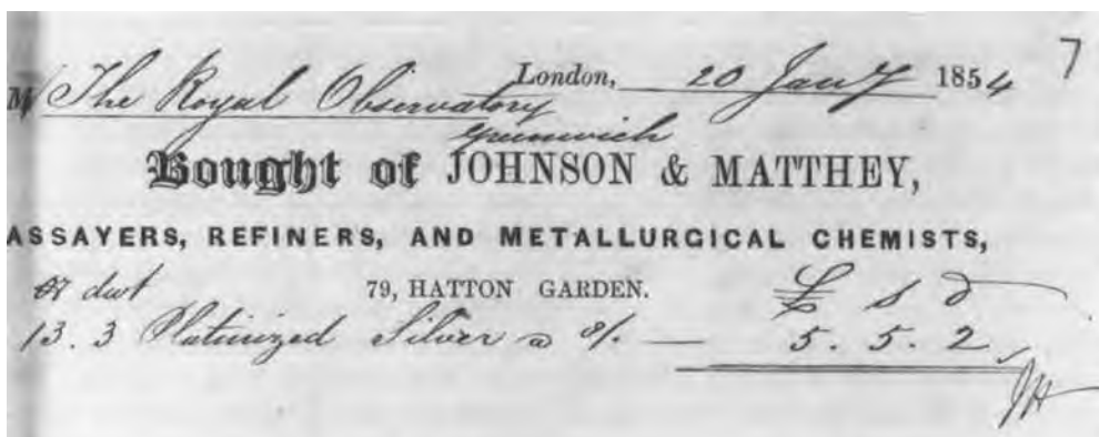
Invoice relating to the supply by Johnson & Matthey of sixty platinised silver plates required by Airy in the manufacture of Smee batteries to be used for transmitting his Greenwich time-signals. The plates measured five by three inches, and were about 0.0026 inches thick
