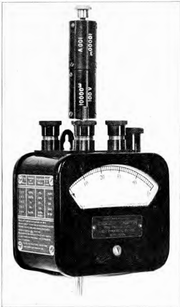
FIG. 4.—DETECTOR WITH BOTH MULTIPLIERS FITTED ON TERMINAL 3.
