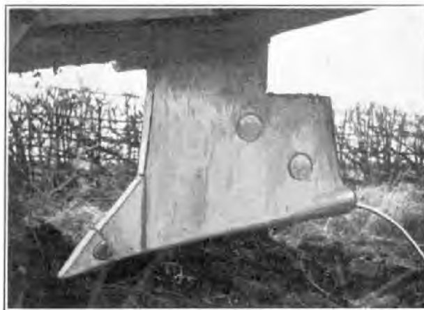
FIG. 5.—RIPPER BLADE WITH CABLE-LAYING MODIFICATION.
