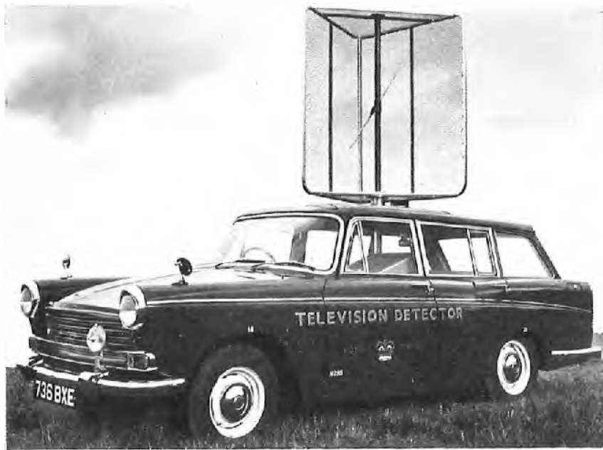
FIG. 1—DETECTOR CAR AND AERIAL
