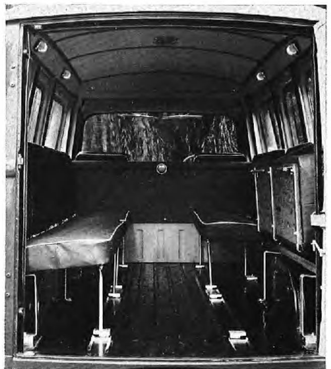
FIG. 6.—INTERIOR OF 15 CWT PERSONNEL CARRIER
