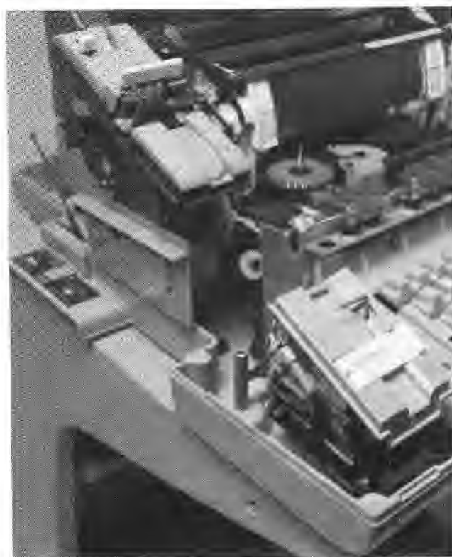
FIG. 7—Paper-tape reader and punch units
