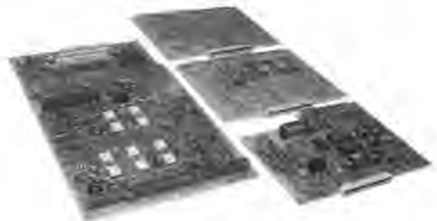
FIG. 6—Printed-wiring boards used in Teleprinter No. 23
