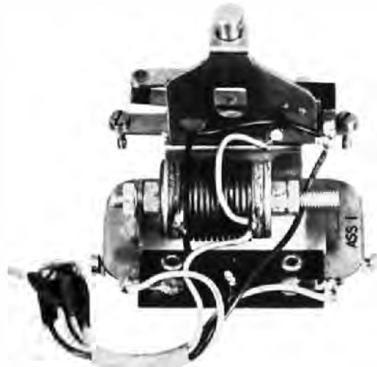
Fig. 3 : The adapter, which comprises the extra key, rectifier and thermistor necessary to convert the telephone for use on automatic shared service systems
