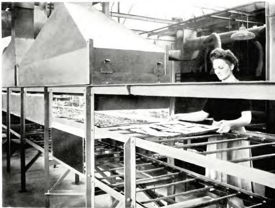
Fig. 3—Parts being fed on to the Conveyor of the Infra-Red Dryer
