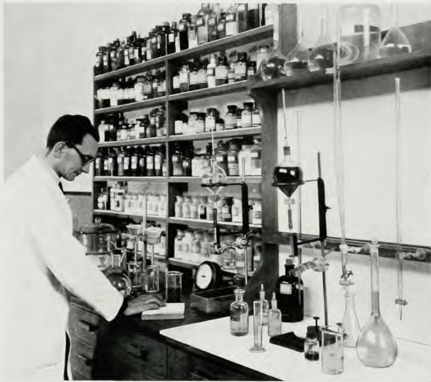
Fig. 2—Control and Testing of Electro-plating Solutions and Deposits
