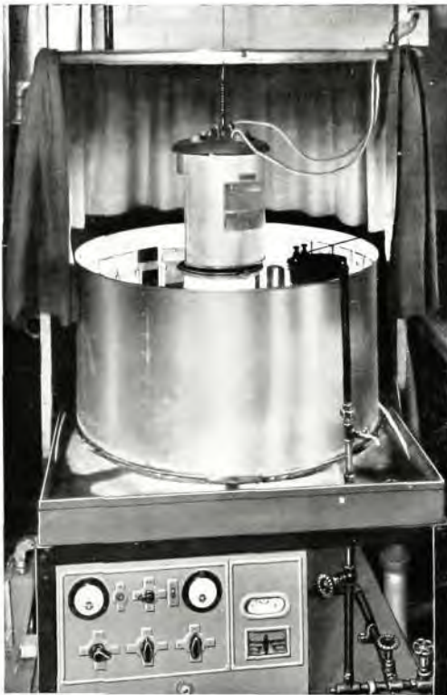
Fig. 1—Accelerated Weathering of Specimen Panels
