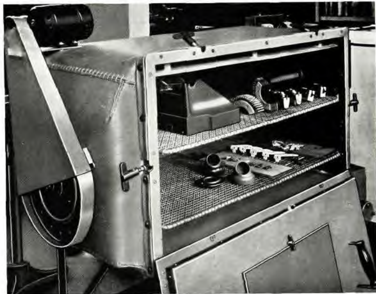
Fig. 4—Components undergoing Tropical Humidity Tests
