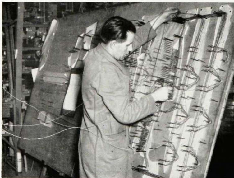
Fig. 1—The laying of a rack cable for a P.B.X. apparatus rack
