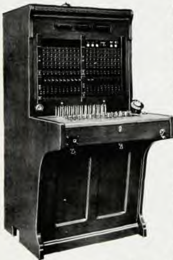
South Africa House—Manual Switchboard
