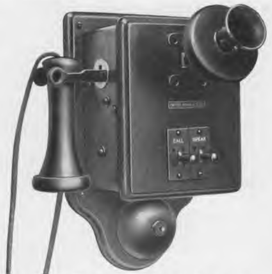
Fig. 8.—Way station telephone (wall pattern).
