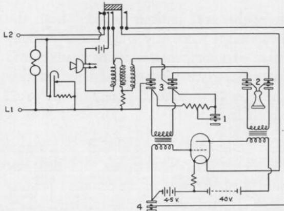
Fig. 2.—Circuit for magneto telephone combined with battery-operated amplifier.
