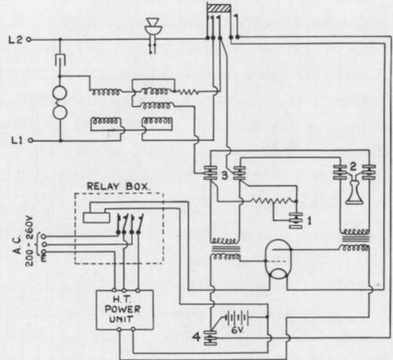
Fig. 5.—Circuit for combined amplifier and C.B. telephone with power unit.
