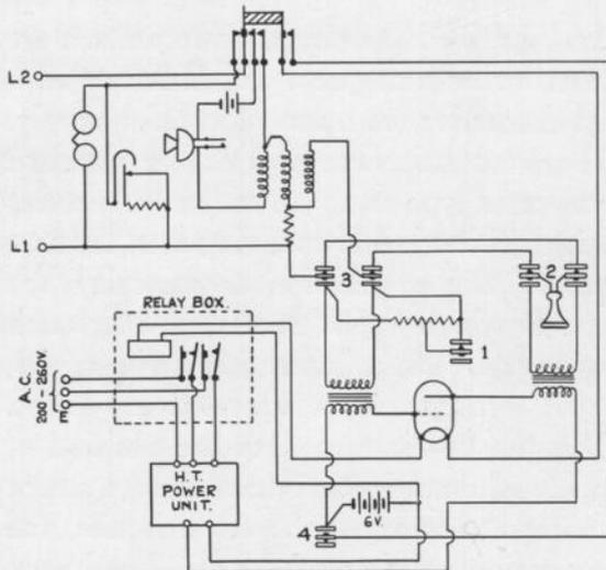
Fig. 4.—Circuit for combined amplifier and magneto telephone with power unit.
