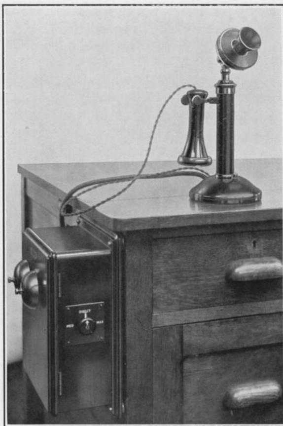
Fig. 1.—Amplifier combined with C.B. telephone.
