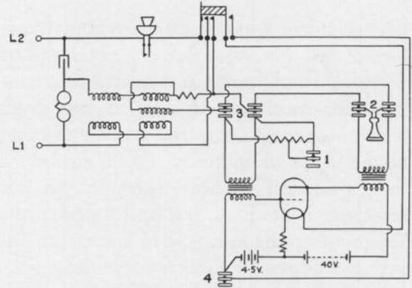
Fig. 3.—Circuit for C.B. telephone combined with battery-operated amplifier.
