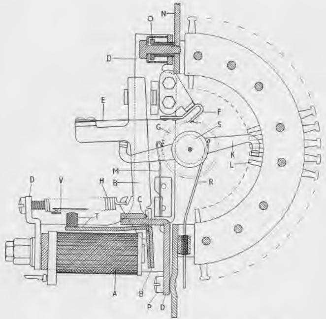
Fig. 4. Control station selector—mechanical details.
