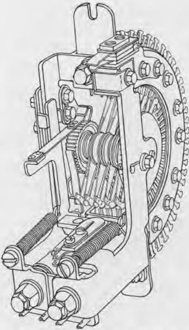
Fig. 3. Control station rotary selector.
