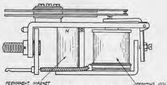
Fig. 2. Polarised line relay.
