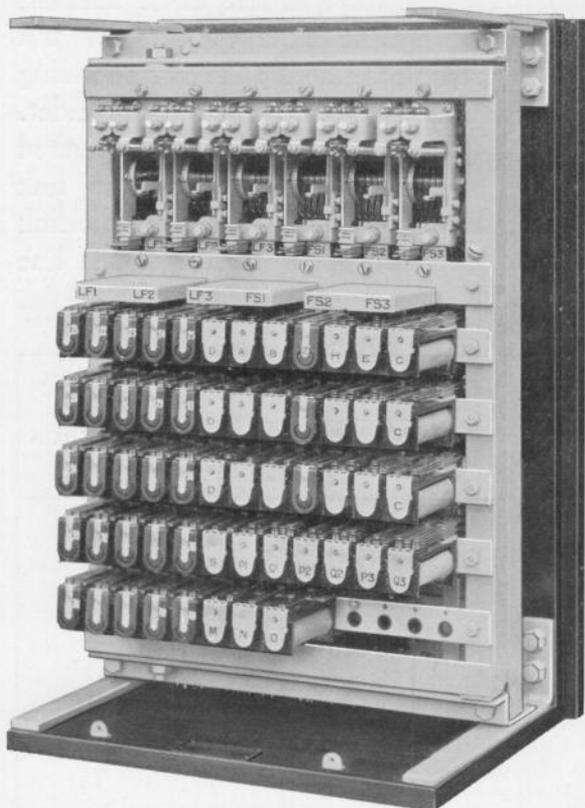
Fig. 2.—Cat. No. 5125 25-line P.A.X. (wood cover removed).
