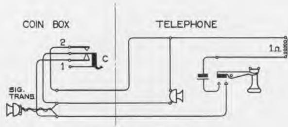
Fig. 9.—Schematic circuit of Postpayment Coin Collector.
