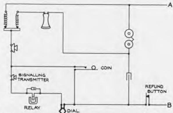
Fig. 7.—Simplified circuit arrangements when employed on an automatic system.
