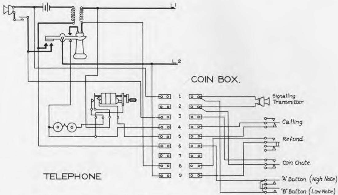
Fig. 8.—Circuit arrangement of Two-Button Prepayment Coin Collector for magneto systems.
