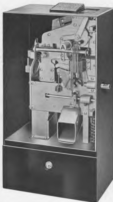
Fig. 2.—Cover removed for inspection of mechanism.
