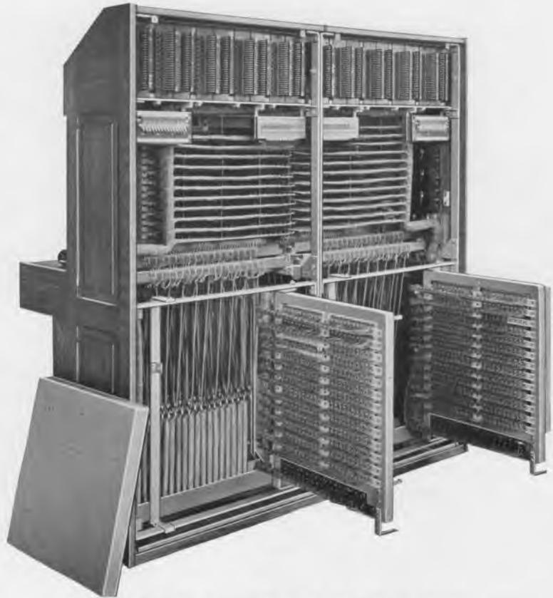
Fig. 2.—Rear doors removed, showing hinged relay frames.
