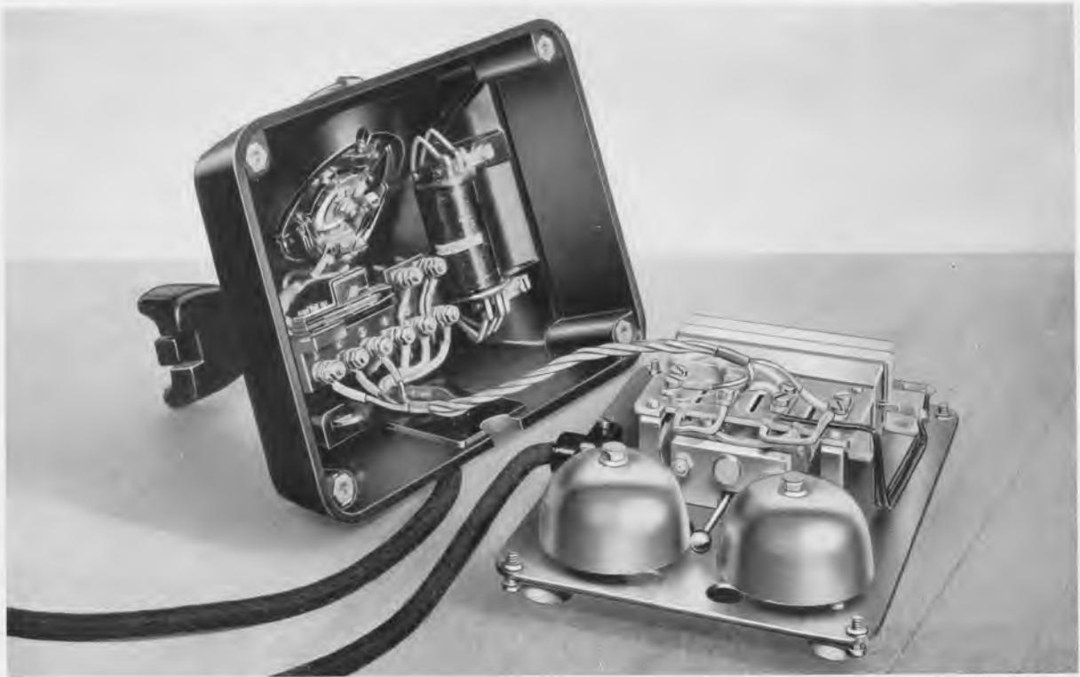
Fig. 3. Instrument open for inspection, giving direct access to every component.
