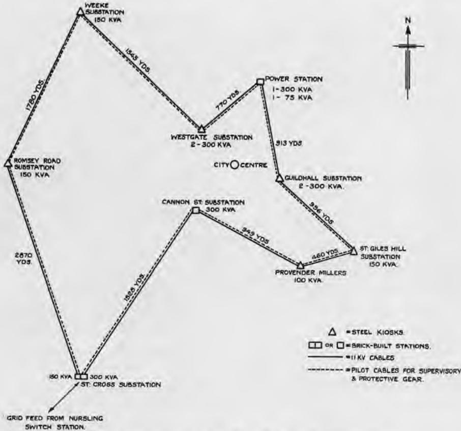
Fig. 1.—A.C. Distribution System of the Winchester Corporation.
