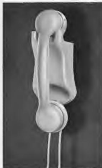
Fig. 1.—Telephone Instrument for use in Flats.
