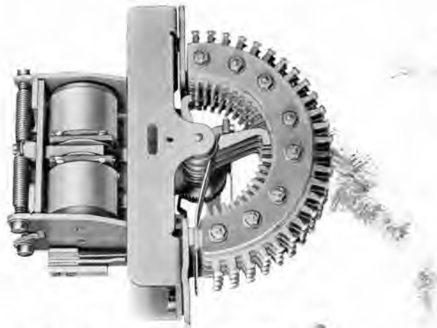
Fig. 1.—Both-way Uniselector, showing coils.
