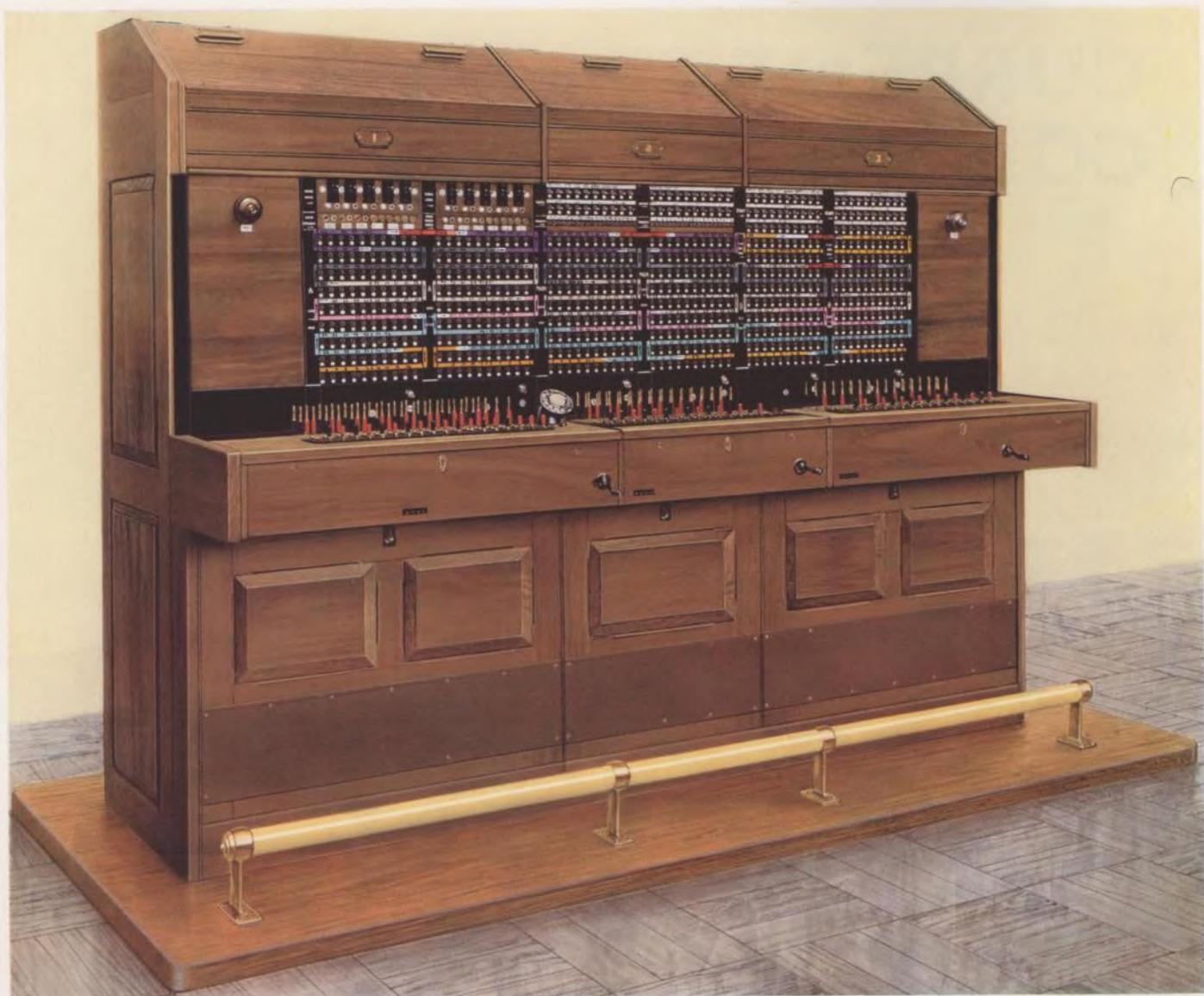
**C.B. Lamp-Signalling Switchboard specially designed for the S.S. *Queen Mary*.**
