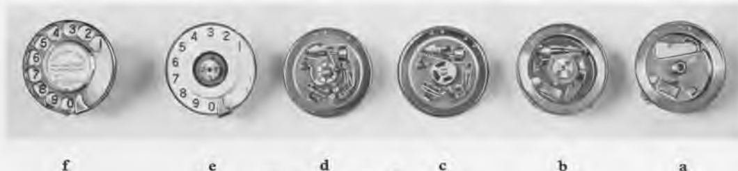
Fig. 8.—Stages of assembly.
