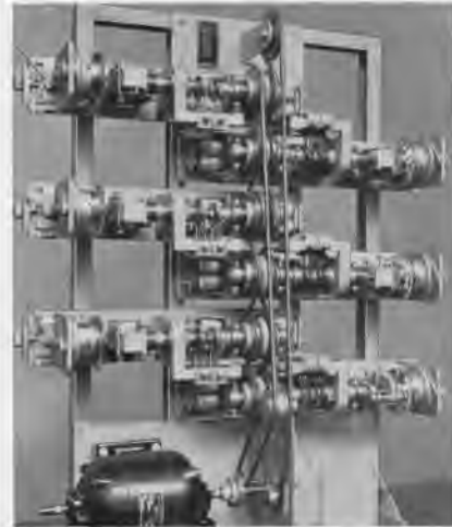
Fig. 9.—Dials under life test.
