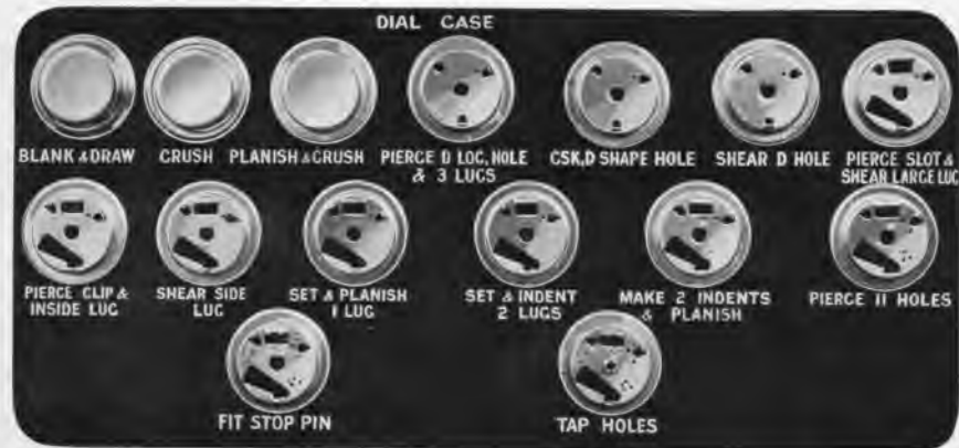
Fig. 3.—Successive stages in the production of the case.
