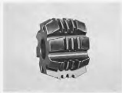
Fig. 5.—Special hob for cutting star wheel teeth.
