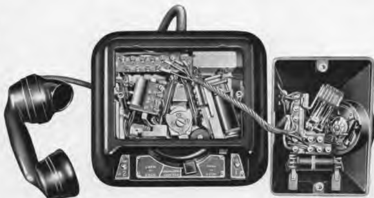
Fig. 3.—Interior of Switching Telephone.
