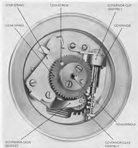
Fig. 3.—Driving mechanism.
