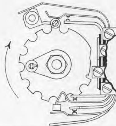
(c) Impulsing position ; trigger moved into engagement with impulse springs.
