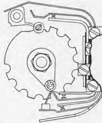
(a) Normal position ; trigger lying under impulse springs.
