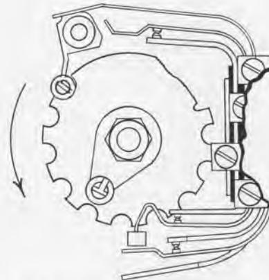
(b) Articulated position ; trigger moved by impulse wheel away from impulse springs ; off-normal springs actuated.
