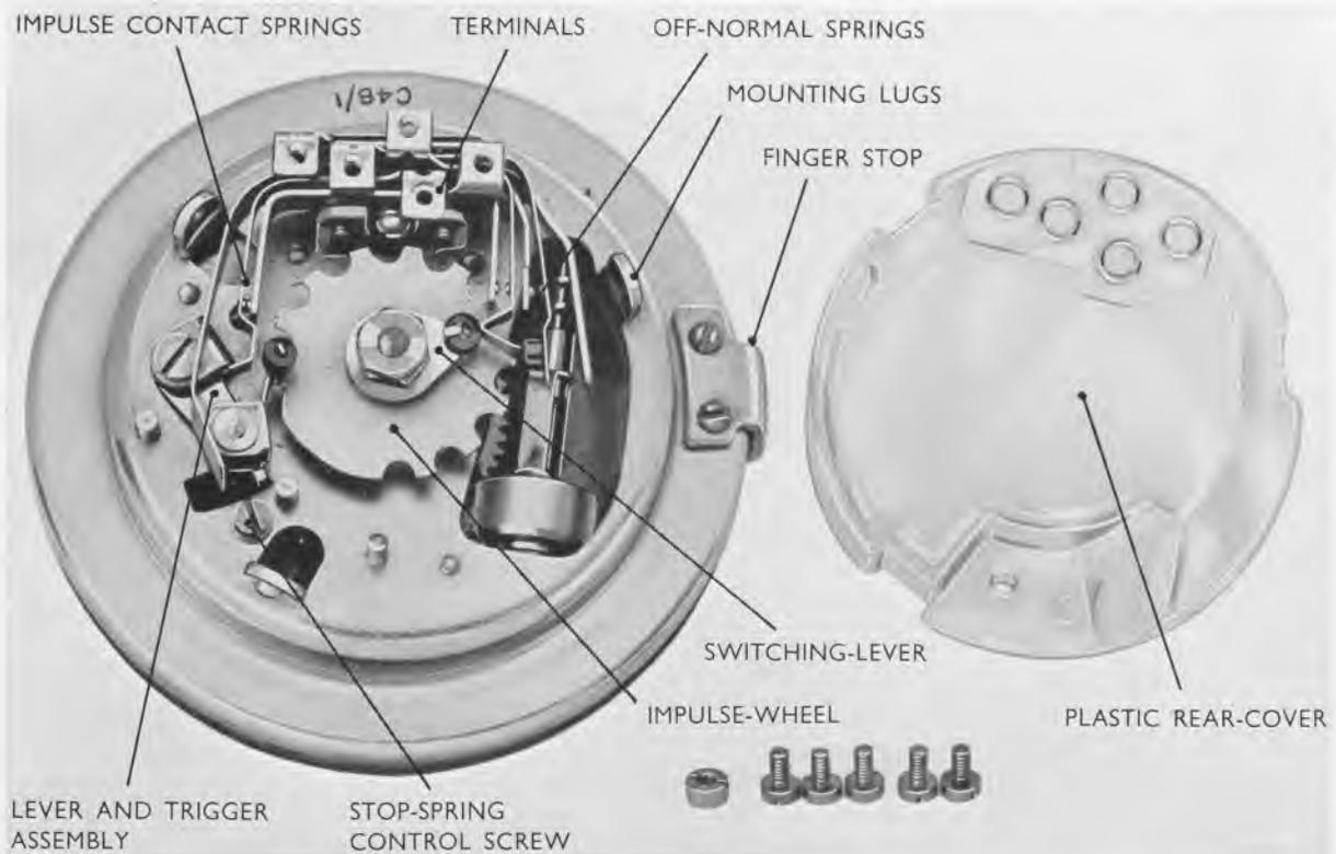
Fig. 1.—Rear view of Dial—with components identified.
