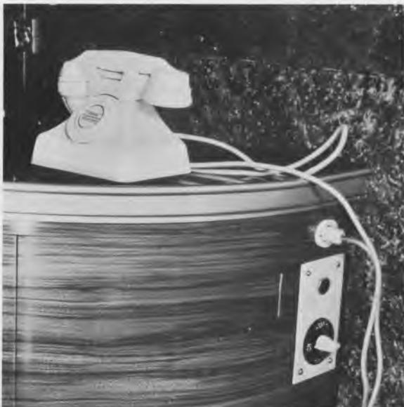
Fig. 5.—Plug and socket connexion for alternative positions of Gecophone to suit passenger convenience.
