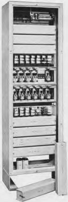
Fig. 1.—2+23-line P.A.B.X. with doors removed.
