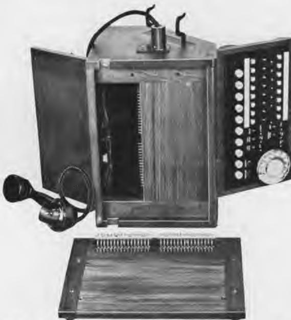
Fig. 4.—10 + 49-line P.A.B.X.—attendant's cabinet with keyboard and backboard open and base removed.
