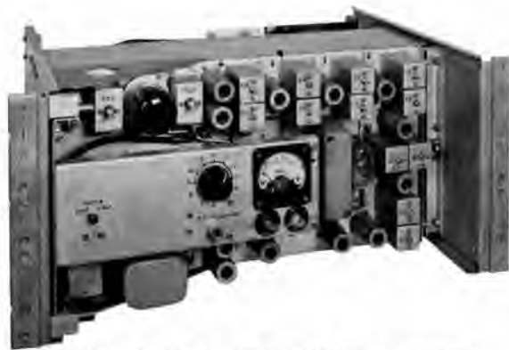
Fig. 12.—Front view of FM VHF link transmitter BRT 143 with cover removed.
