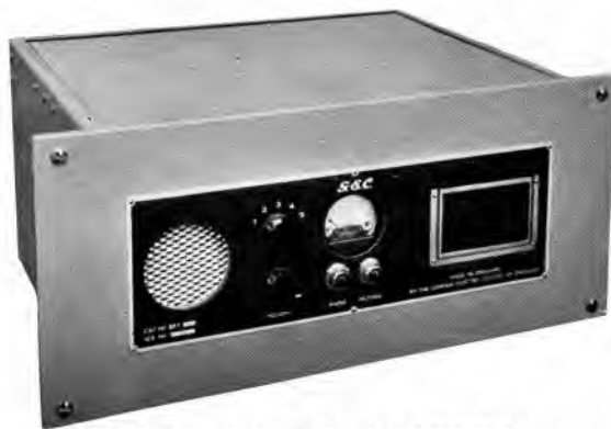
Fig. 2.—Front view of typical VHF link receiver, BRT 186.
