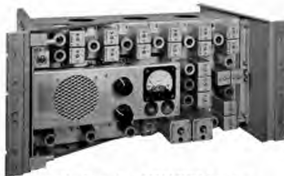
Fig. 13.—Front view of FM VHF link receiver BRT 163 with cover removed.
