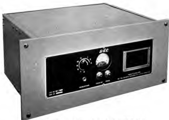
Fig. 1.—Front view of typical VHF link transmitter, BRT 143.
