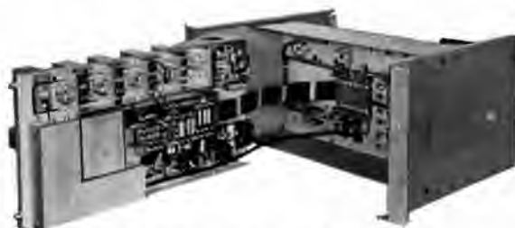
Fig. 9.—FM receiver BRT 163 with RF chassis swung open for inspection.
