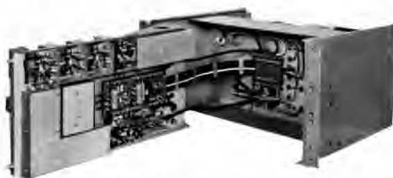
Fig. 8.—FM transmitter BRT 143 with RF chassis swung open for inspection.
