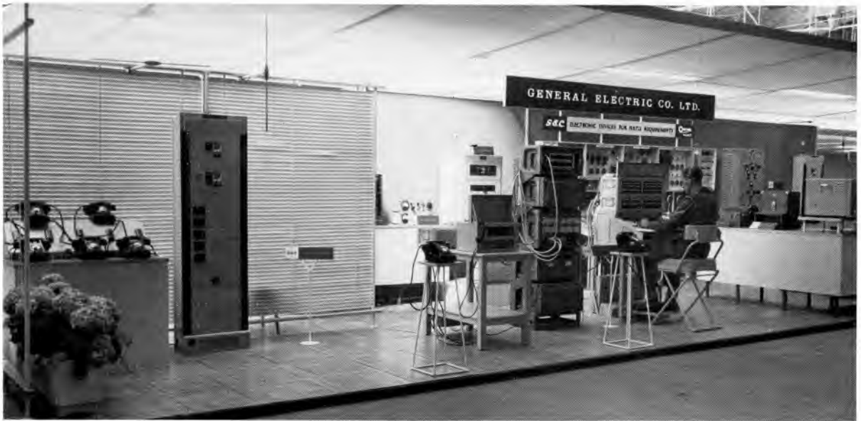
A general view of the G.E.C. stand showing a 5-circuit VHF Junction Radio Terminal on the left and the Manual Exchange CB20 on the right.
