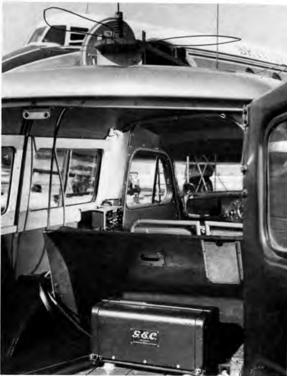
Fig. 1.—A mobile VHF transmitter/receiver installed in a vehicle as a mobile extension of London Airport telephone exchange.
