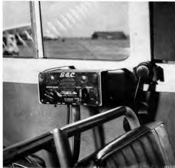
Fig. 1.—A mobile VHF transmitter/receiver installed in a vehicle as a mobile extension of London Airport telephone exchange.
