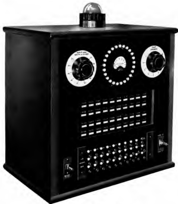
Fig. 3.—Supervisor's control cabinet.
