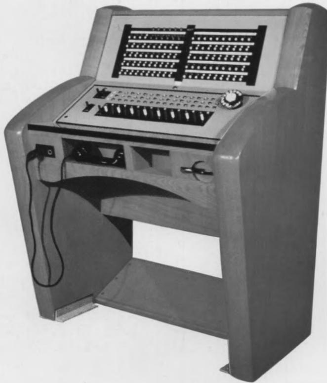
*Her Majesty's Yacht Britannia has been equipped with the first of the latest C.B. cordless telephone exchange designed by the G.E.C. The exchange combines the advantages of both cord and cordless switchboards. Ease of operation is ensured by pushbutton operation, whereby the operator initiates selection processes through automatic apparatus. Identification of calling lines is provided by coloured line lamps.*
