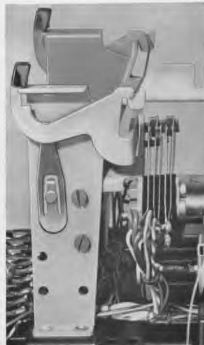
Fig. 7.—Cradle switch held operated by spring clip.
