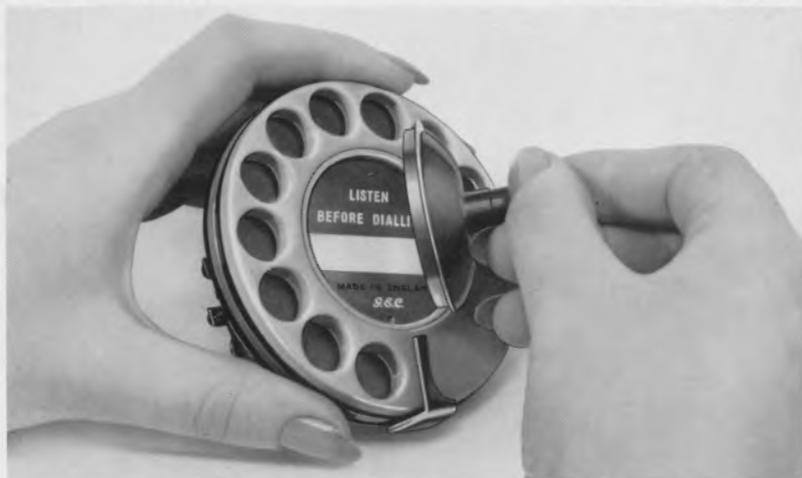
Fig. 4.—Illustrating removal of protector with rubber suction pad.
