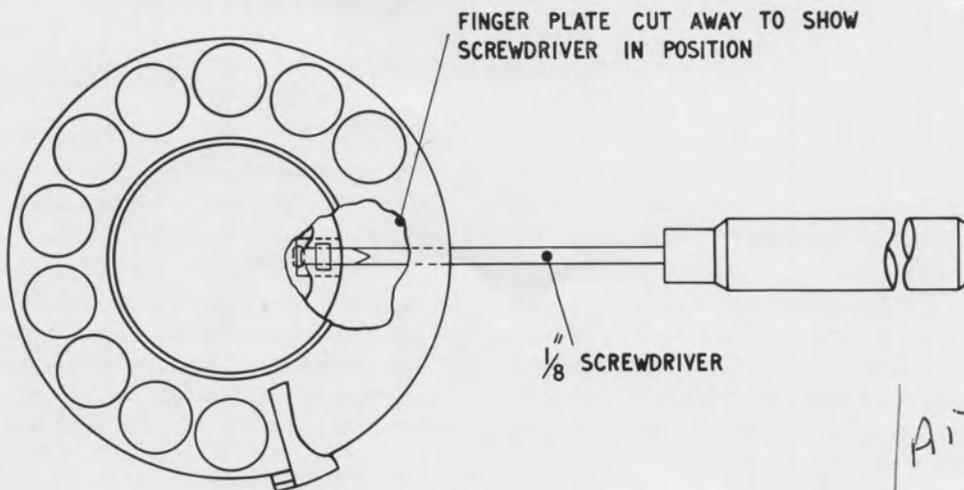
Fig. 5.—Illustrating removal of protector with screwdriver.
