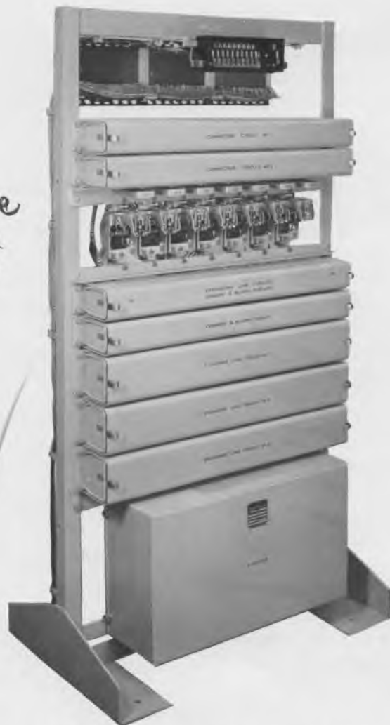
Fig. 6.—3 + 10-line P.A.B.X. with cabinet removed.
