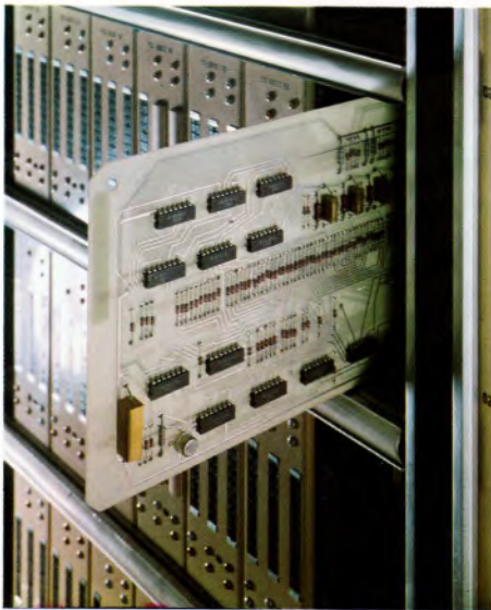
Extensive use is made of printed circuit boards and integrated circuits, for economy of space and maintenance.
