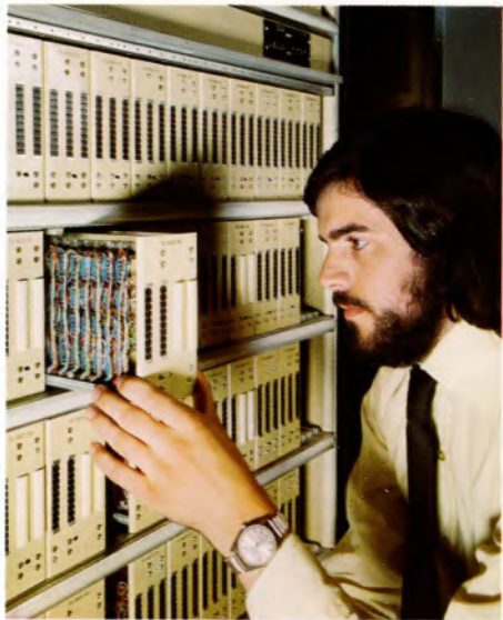
Plug-in modules make for ease of maintenance and simple extension of the service.
